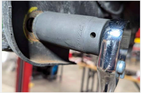
Figure 1: Lower A-Arm bolt Removal
