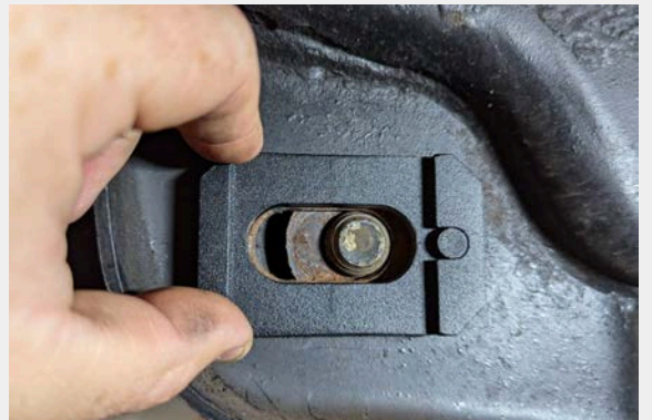
Figure 4: Guide Plate Installed
