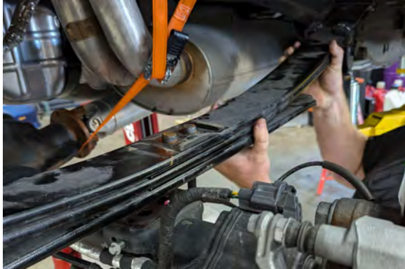
Figure 11: Leaf Spring Install
