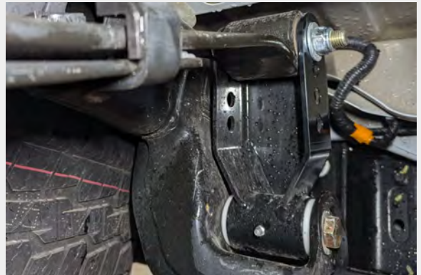
Figure 13: Installed Adjustable Leaf Spring Shackle
