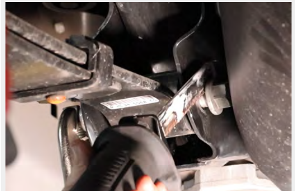
Figure 4: Cut Front Spring Mount Bolt
