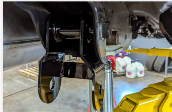
Figure 10: Installed Front Leaf Spring Mount
