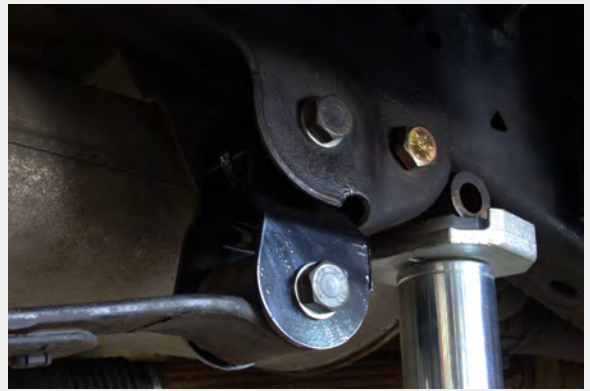
Figure 12: Installed Front Leaf Spring Mount
