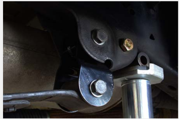
Figure 27: Installed Front Leaf Spring Mount
