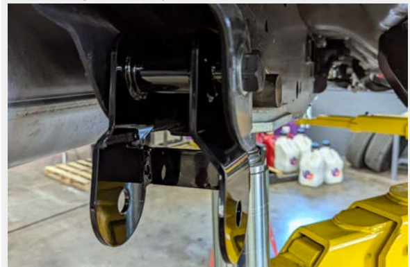
Figure 25: Installed Front Leaf Spring Mount
