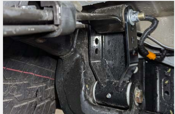
Figure 28: Installed Adjustable Leaf Spring Shackle
