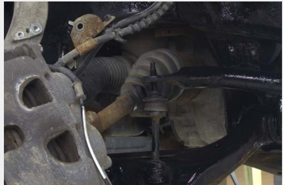
Figure 2: Sway Bar End Link Removal
