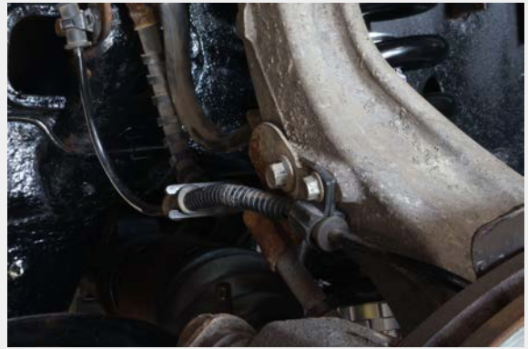
Figure 1: ABS Cable Removal
