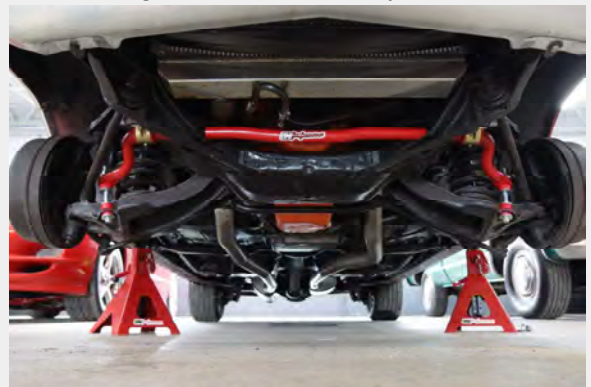
Figure: Finish Installed Sway Bar
