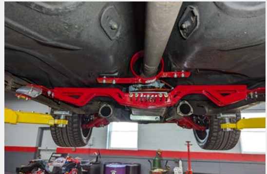
Figure 6: Fully Installed Crossmember
