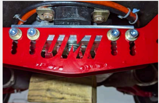
Figure 5: Adjustment Block Installed
